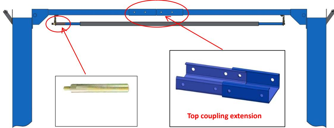
5、Connect the extension hose with the fitting and install the extension small cable:
