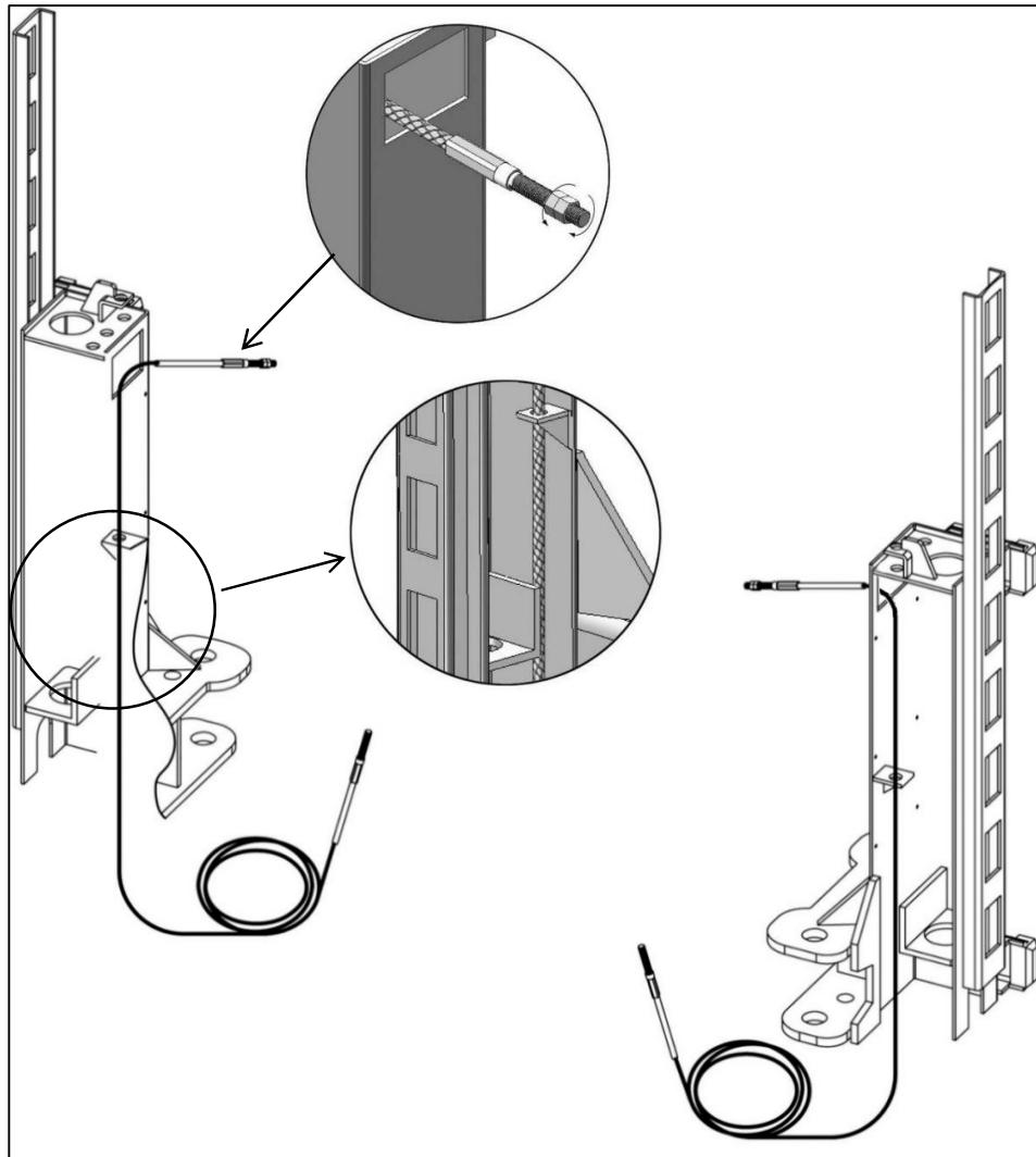
4、Install the Top coupling extension kit and install the control rod extension pin:
