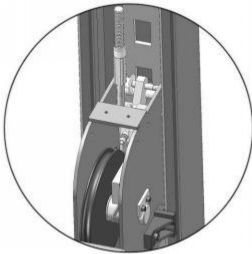
Cable pass through between the big pulley and tension pulley D View Fig.27
