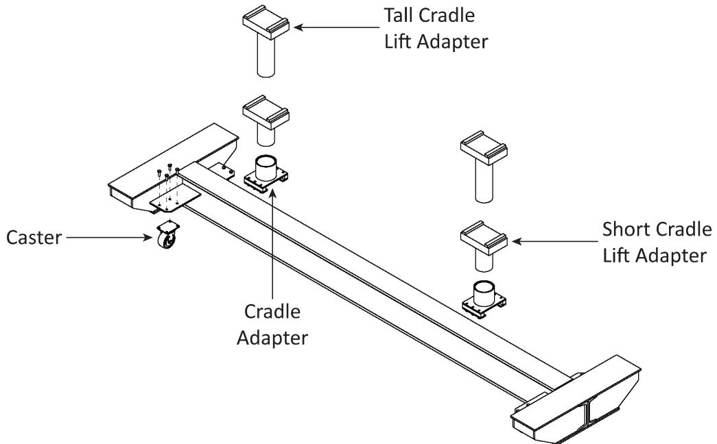
The Crossbeam can support a full 36,000 lbs / 8165 kg for much of its length of 122 inches / 3098.8 mm. However, as the adapters are moved towards the middle of the Crossbeam, the load that can be supported is reduced to a maximum total of 12,950 lbs.
