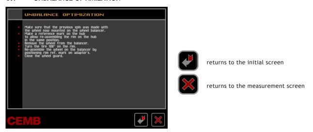
The program allows total wheel out-of-balance to be reduced by compensating, when possible, tyre and rim out-of-balance values. It requires two runs, rotating the tyre on the rim on the second run.
