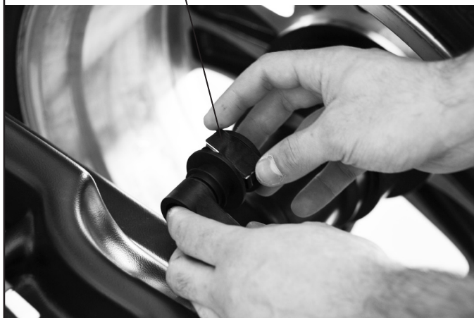
Fig. 33 Fit the adhesive weight in the pliers of the gauge rod
