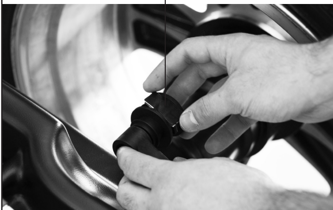
Fig. 27 Fit the adhesive weight in the pliers of the gauge rod
