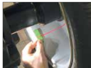
Quick selection and rim run-out measurement with internal data gauge.
