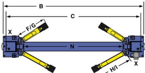
NOTE: Power unit can be located at either X location.
